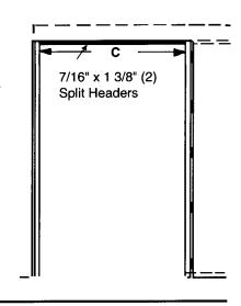
Open door fully (door will protrude into opening) and cut split jambs to "B". Fasten to front edge of frame. Maintain minimum 3/16" clearance on both sides of door. Raise or lower hangers to plumb door with split jambs.
